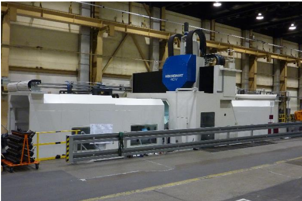
Fig. 3. Machining center with the possibility of working displacement in axes: X = 14,700 mm, Y = 4,000 mm and Z = 2,050 mm
