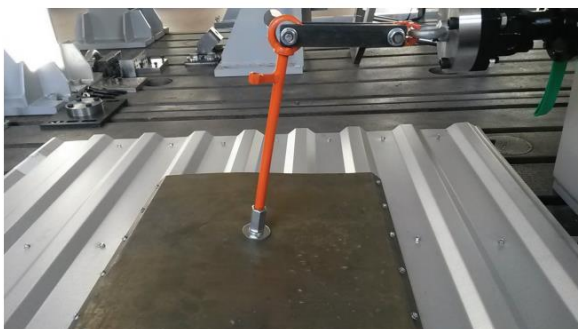
Fig. 8. Study of the construction in a direction perpendicular to the trapezoidal sheet piles
