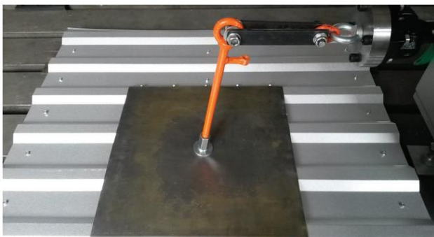
Fig. 9. Study of the construction in parallel direction to the trapezoidal sheet piles
