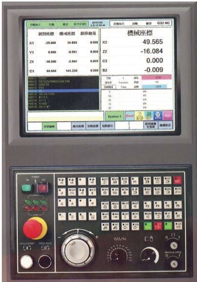
Fig. 3. CNC L2100 type controller developed by ITRI (source: www.itri.org.tw/eng )
