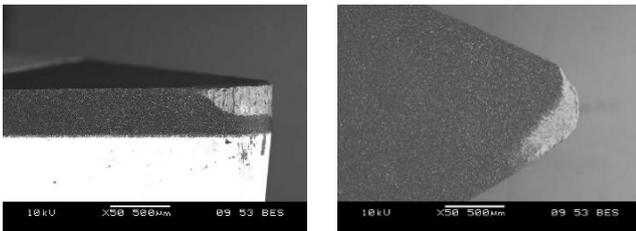
Fig. 10. PCD tools after turning AK7-SiC material: a) surface of application, b) rake surface (cutting speed: 500 m/min, feedrate: 0.10 mm/rev, depth of cut: 0.5 mm)
