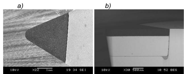
Fig. 5. Polycrystalline diamond plate marked NP-DCMW11T304 MD220: a) rake surface, b) grinding surface and cutting edge
