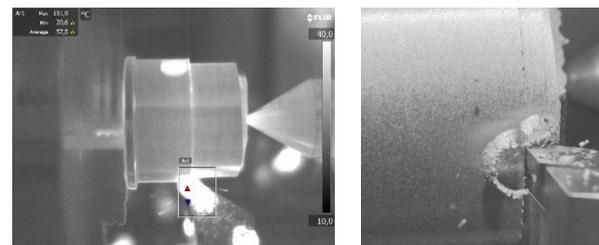
Fig. 7. Thermal imaging camera image (a), chip forming mechanism (b) (cutting speed: 45 m/min, feedrate: 0.34 mm/rev, depth of cut: 2 mm)
