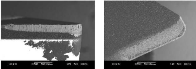
Fig. 11. PCD tools after turning AK7-SiC material: a) surface of application, b) rake surface (cutting speed: 500 m/min, feedrate: 0.20 mm/rev, depth of cut: 2.0 mm)
