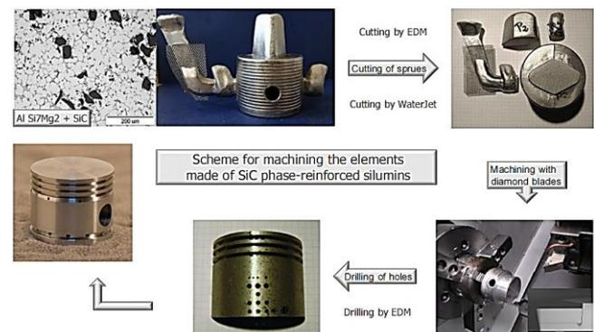
Fig. 1. Silicon carbide SiC reinforced machining scheme
