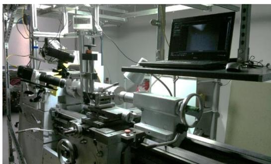
Fig. 3. Apparatus for temperature measurement and analysis of chip formation mechanism during turning
