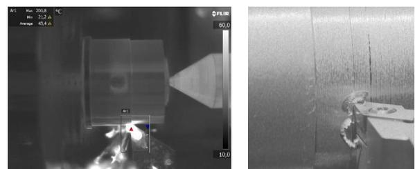
Fig. 9. Thermal imaging camera image (a), chip forming mechanism (b) (cutting speed: 120 m/min, feedrate: 0.34 mm/rev, depth of cut: 1 mm)
