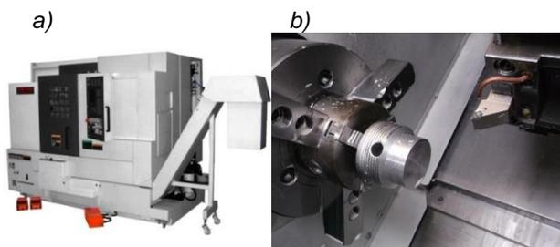
Fig. 2. Position NL2000SY for cutting tests (a), view of machining system: handle - workpiece (piston) - tool (b)
