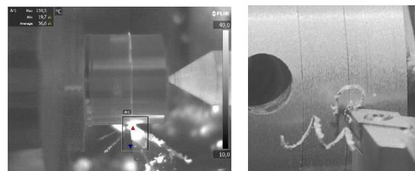
Fig. 8. Thermal imaging camera image (a), chip forming mechanism (b) (cutting speed: 100 m/min, feedrate: 0.34 mm/rev, depth of cut: 0.5 mm)
