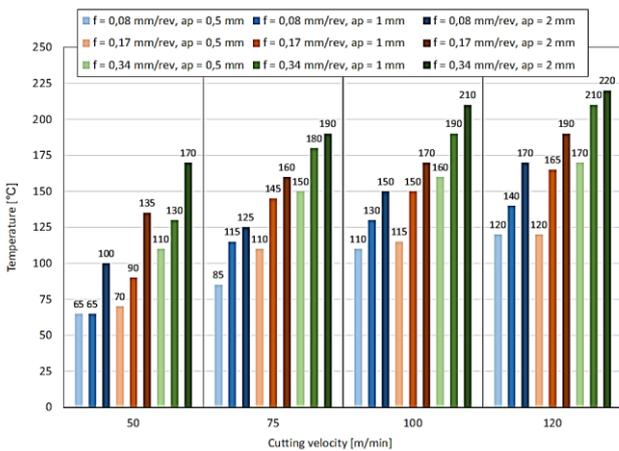
Fig. 6. Effect of cutting parameters (velocity  $v_c$ , feed  $f$ , depth  $a_p$ ) on polycrystalline diamond blade temperature value
