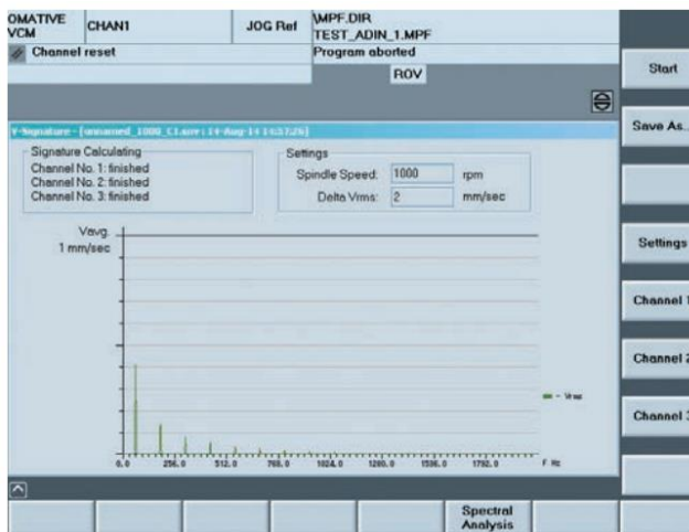
Fig. 4. Screen appearance of NC controller with VCM spectra measurement results for spindle vibrations (www.omative.com)
