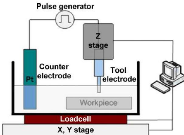
Fig. 5. Schematic diagram for SACE (spark assisted chemical engraving) workbench in drilling and milling kinematics [10]
