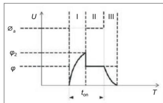
Fig. 2. Typical voltage pulse waveform in ECDM; Phase I - increase of inter-electrode voltage with simultaneous electrochemical phase of electrochemical dissolution and hydrogen secretion up to the attenuation voltage  $\phi_2$  and spark initiation. At the start of the discharge the voltage drops to  $\phi$  - Phase II, where the arc discharge lasts until the end of the voltage pulse; Phase III, as a result of the capacitive effect, the voltage gradually decreases to zero [9]
