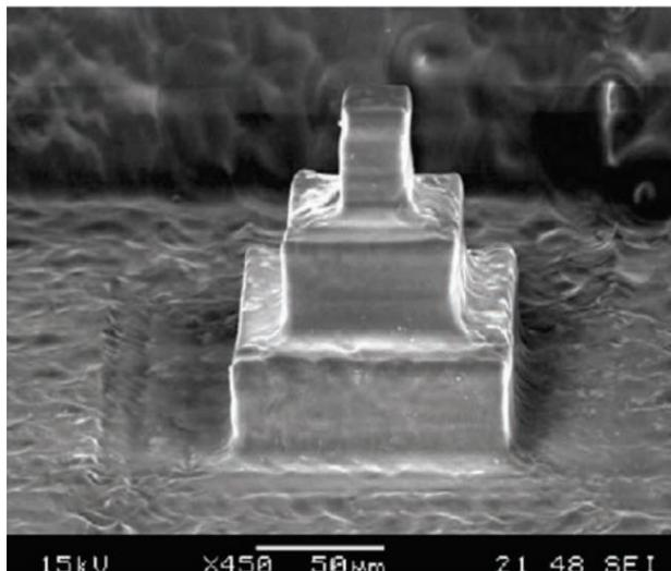
Fig. 9. Micro-pyramid made by milling in Pyrex Glass by SACE method. Machining parameters: 30% KOH,  $U = 23\ \text{V}$ , pulse/pause time  $1\ \text{ms}/1\ \text{ms}$ , tool diameter  $30 \div 33\ \mu\text{m}$ , feedrate  $3\ \mu\text{m/s}$ , tool rotation  $300\ \text{rpm}$ ; Roughing:  $U = 28\ \text{V}$ , KOH 30%, pulse time/pause time  $1\ \text{ms}/1\ \text{ms}$ , feedrate  $3\ \mu\text{m/s}$ . Total processing time 3 hours. [10]
