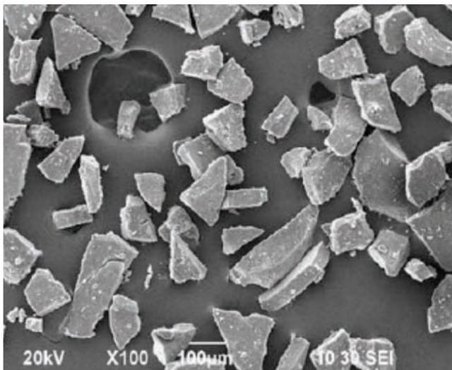
Fig. 3. ECDM erosion products in 359 aluminum alloy reinforced with SiC (voltage amplitude  $U = 110$  V, pulse time 40  $\mu\text{s}$ ,  $\text{NaNO}_3$  electrolyte concentration 1%, current amplitude 5 A, treatment time 3 min, gap between electrodes  $s = 5$  microns). The average size of the largest (percentage) ECDM products varies between  $23 \pm 80$   $\mu\text{m}$  [9]
