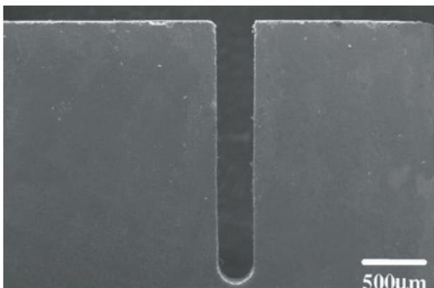
Fig. 10. Width of cutting slit in SACE (Pyrex Glass);  $R_a = 0.84 \mu\text{m}$ , breakage of 0.024 mm, KOH electrolyte with SiC grain size (average particle size  $57 \mu\text{m}$ ) with a concentration of 300 g/l [11]
