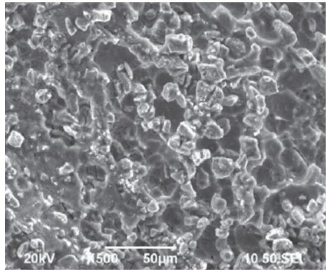
Fig. 4. Typical surface view after ECDM treatment (Al 359 + 20% SiC grains of 10  $\mu\text{m}$ ) - reusable metallic phase and reinforcing phases and microcracks are visible again [9]
