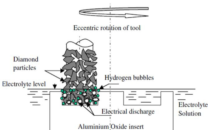
Fig. 11. Schematic diagram of  $\text{Al}_2\text{O}_3$  element machining with SACE electrodes with abrasive grains [12]
