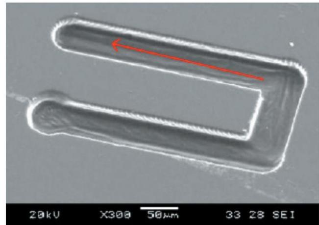
Fig. 7. Cavity made in Pyrex Glass during milling operation: feedrate  $3\ \mu\text{m/s}$  (30% KOH,  $23\ \text{V}$  breakout voltage,  $1\ \text{ms}/1\ \text{ms}$  pulse/break time). Surface roughness:  $R_a = 0.099\ \mu\text{m}$  [10]
