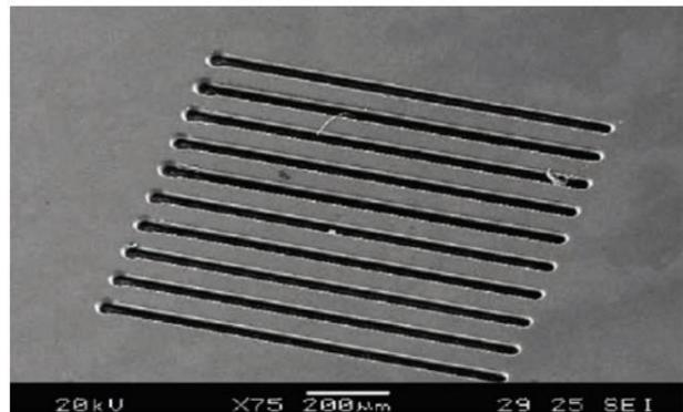
Fig. 8. Microwaves made by the SACE method: 30% KOH,  $U = 23\ \text{V}$ , pulse time/break time  $1\ \text{ms}/1\ \text{ms}$ , tool diameter  $30 \div 33\ \mu\text{m}$ , feedrate  $3\ \mu\text{m/s}$ , tool rotation  $300\ \text{rpm}$ . Pyrex Glass workpiece, dimensions: depth  $30\ \mu\text{m}$ , length  $1000\ \mu\text{m}$ , width  $40\ \mu\text{m}$ . Processing time of each slot  $360\ \text{s}$  [10]
