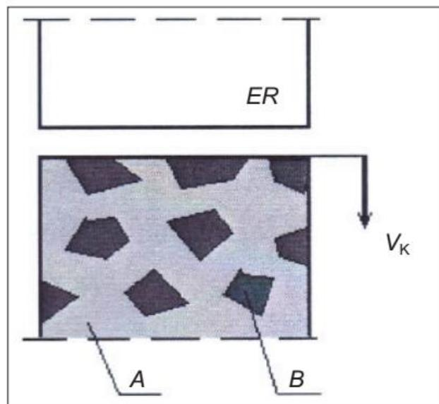
Fig. 1. Machining the workpiece made of composite material. A - matrix material (metal or ceramic material), B - reinforcement phase particles (metal or ceramic grain), ER - working electrode
