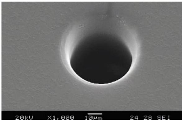
Fig. 6. Micro-hole ECDM drilling in glass plate (Pyrex Glass)  $150\ \mu\text{m}$  thick. Tool diameter  $31\ \mu\text{m}$ , 30% KOH electrolyte,  $U = 30\ \text{V}$ , pulse time = break time =  $1\ \text{ms}$ , tool rotation  $300\ \text{rpm}$  [10]
