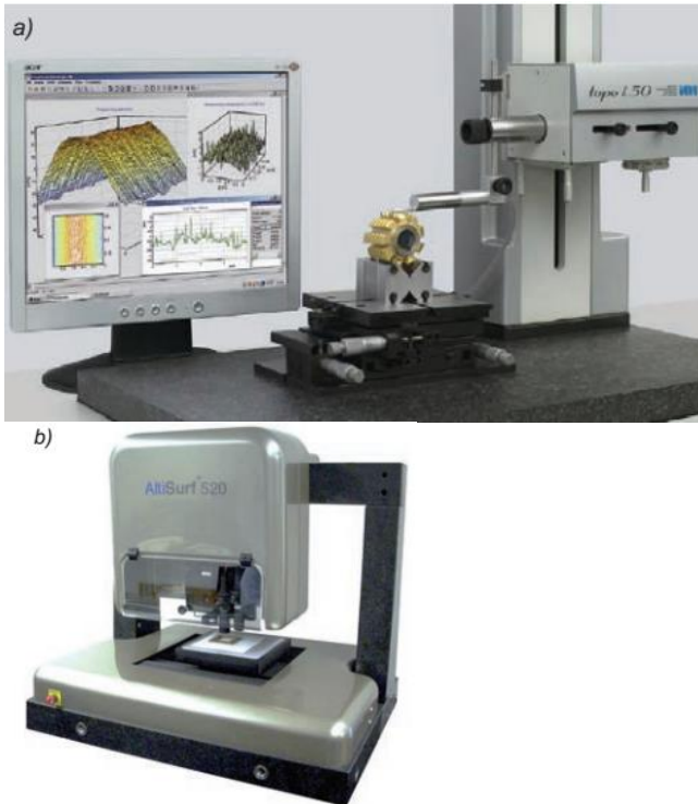
Fig. 1. TOPO 01P contact profilometer (a) and AltiSurf 520 optical system (b)
