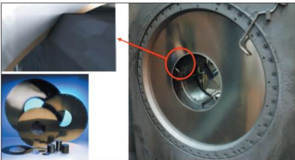
Fig. 3. Disc with internal cutting edge, used for abrasive cutting [13, 19]
