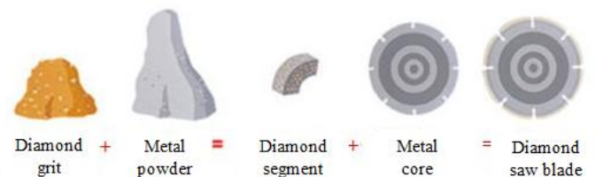
Fig. 1. The idea of forming an abrasive diamond disc [14]
