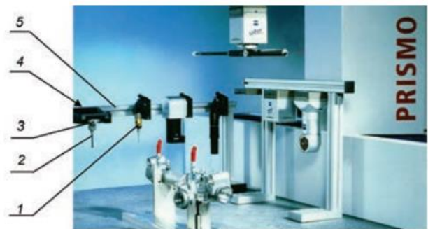
Fig. 4. Frame of heads and measuring spindles (tips): 1 - one of the measuring heads, 2 - measuring spindle, 3 - fixing plate, 4 - socket, 5 - socket mounting frame
