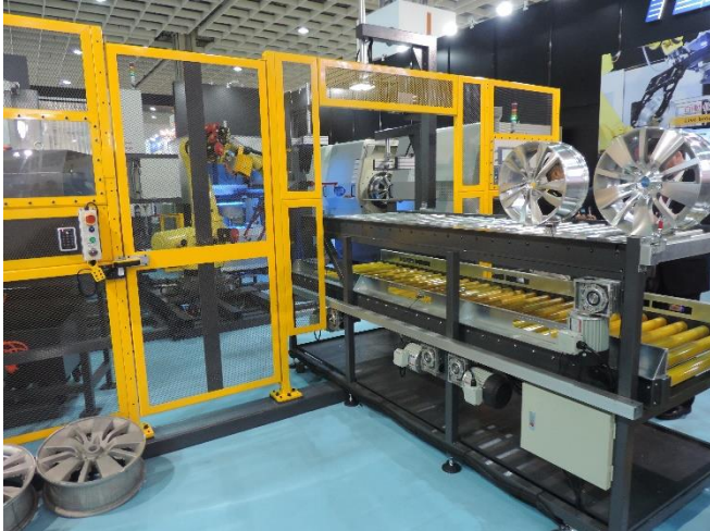
Fig. 3. FEMCO machined line for machining aluminum rims
