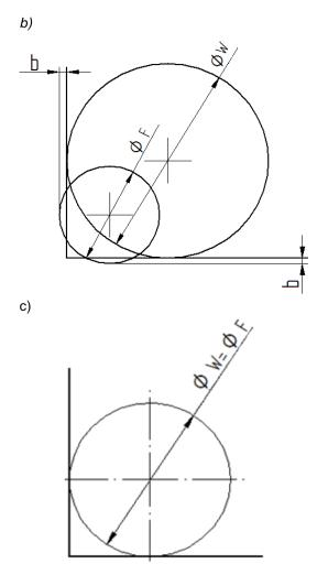
Fig. 2. Tested cases: a)  $\emptyset$  drill bits <  $\emptyset$  milling cutters, b)  $\emptyset$  drill bits >  $\emptyset$  milling cutter, c)  $\emptyset$  drill bits =  $\emptyset$  cutter
