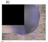
The biggest recess Ø drill bit / Ø cutter= Ø5/ Ø5
