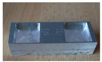
Fig. 1. Sample after roughing - the photo shows different radii of passage in the inner pockets.
