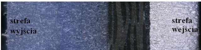
Fig. 3. View of the structure intersection: aluminum alloy 2017A (input zone) - carbon composite - polyamide PA6 (output zone)
