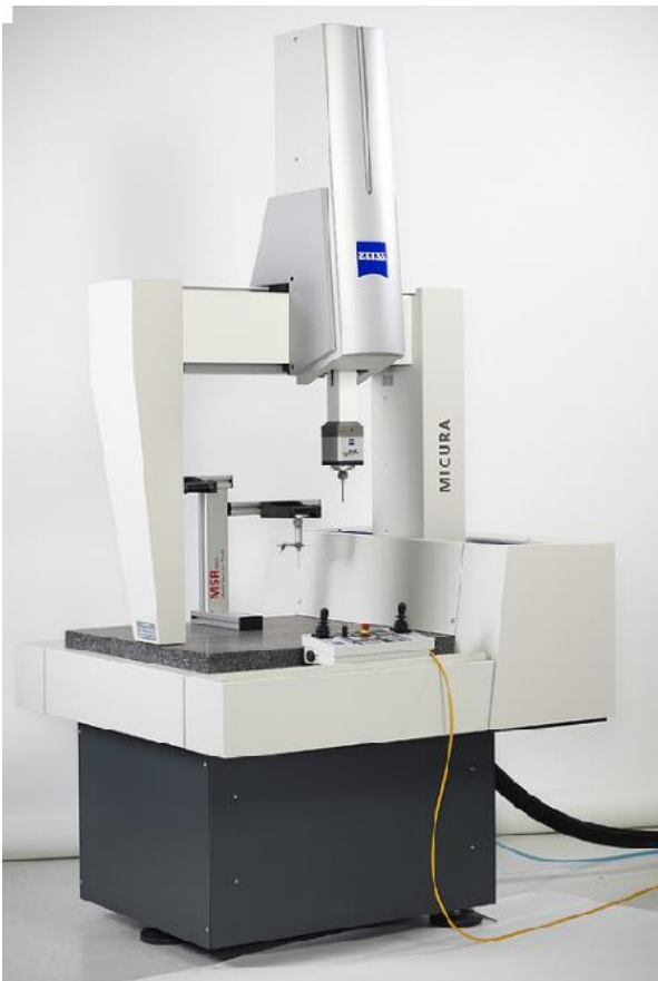
Fig. 3. The Zeiss MICURA portal coordinate measuring machine
