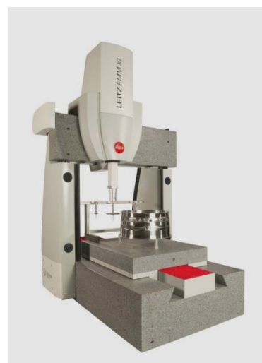
Fig. 5. Coordinate measuring machine Leitz PMM-Xi
