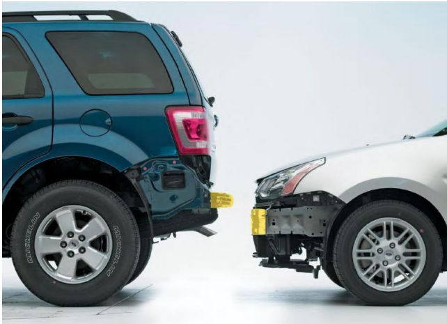
Fig. 6. Different height of bumpers in passenger cars and off-road vehicles is a significant cause of the cost of repairing vehicles after their collisions (source: RCAR [7]).
