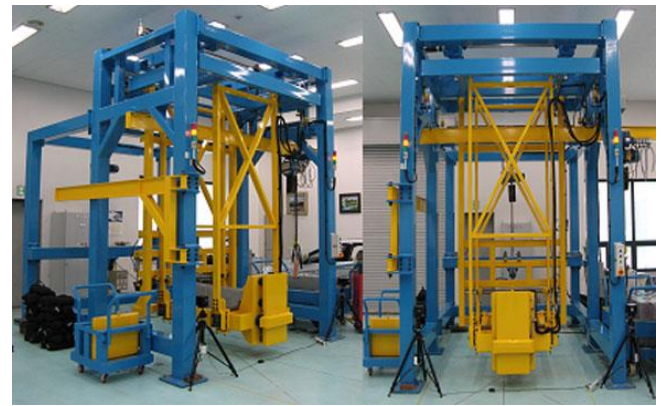
Fig. 4. Pendulum test stand for ECE R42 and FMVSS 581 homologation tests (source: A & G Technology)
