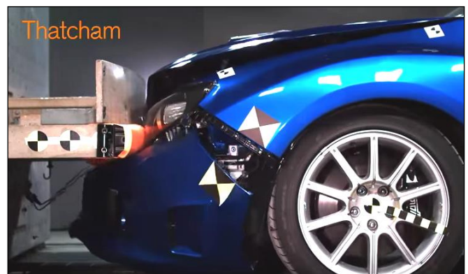
Fig. 1. An example of a frontal impact test at 6 mph by Thatcham. The shock barrier and test procedures defined by RCAR were used for the test. Tested vehicles: a) Toyota Auris, whose accident repair costs were estimated at $ 810; b) Subaru Impreza, whose repair costs amounted to $ 4150 (source: Thatcham)
