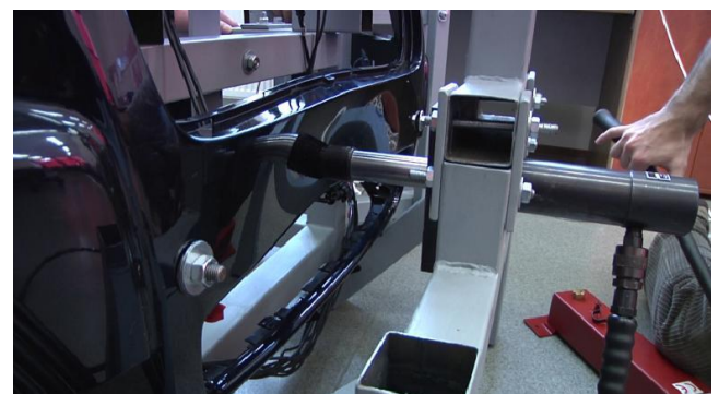
Fig. 8. Use of a hydraulic cylinder to load a car stopper on a stationary test bench
