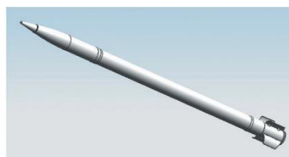
Fig. 1. Solid model of the 122 mm Phoenix missile, developed in the SolidWorks environment
