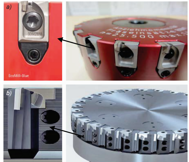
Fig. 19. Chip cutter head with chip dispensing chambers: a) Mapal solution, b) Gühring-Hollfelder solution
