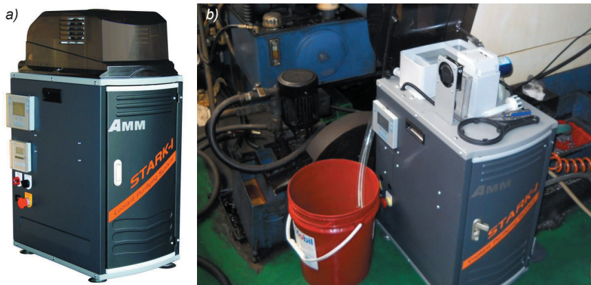
Fig. 7. Sample cooling unit [3] (a), machine combined with cooling system [1] (b)
