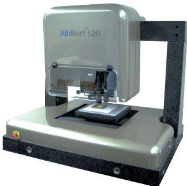
Fig. 1. Altisurf 520 profilometer of modular design for optical and contact measurements
