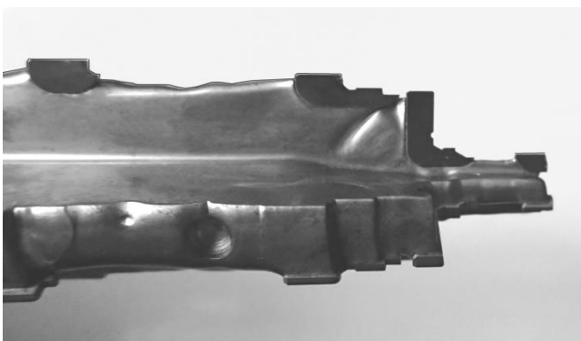
Fig. 12. Traces on the tool body due to diamond-tipped blades after processing several hundred thousand objects (according to Mapal)
