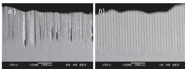
Fig. 7. Cross-sectional SEM micrographs of SL of Vanadis 6 steel samples subjected to: a) grinding and b) turning-burnishing
