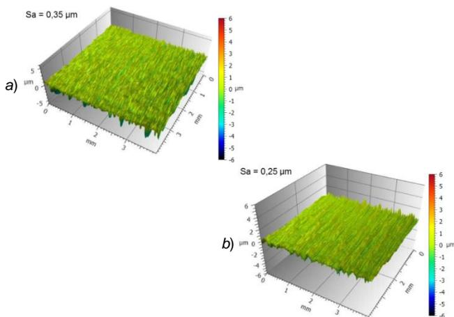
Fig. 5. 3D view of Vanadis 6 steel surface topography after: a) grinding and b) turning-burnishing
