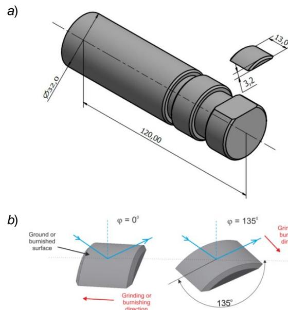
Fig. 3. Dimensions of shafts subjected to mechanical finishing processes (a) and the scheme of stresses measurement in two directions determined by the angle  $\varphi$  (b)
