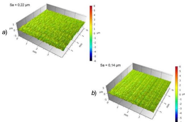
Fig. 4. 3D view of Sverker 21 steel surface topography after: a) grinding and b) turning-burnishing
