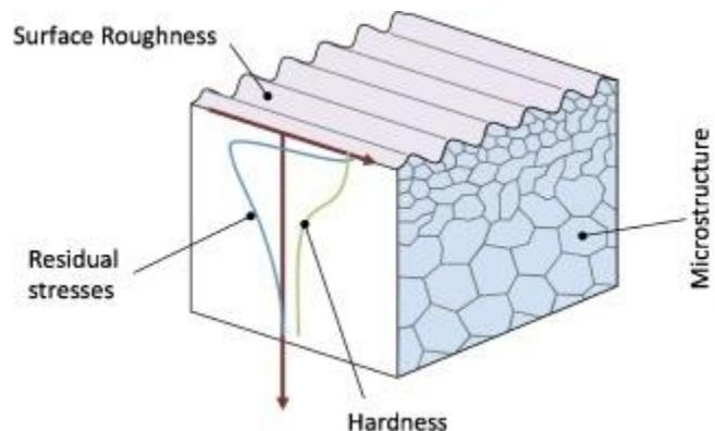
Fig. 1. Selected parameters characterizing the SL according to [4]
