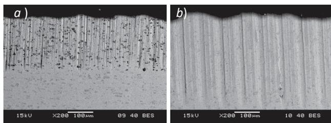
Fig. 6. Cross-sectional SEM micrographs of SL of Sverker 21 steel samples subjected to: a) grinding and b) turning-burnishing
