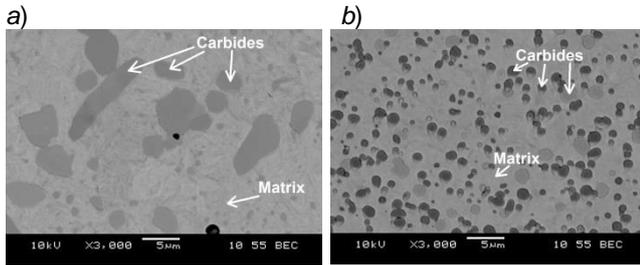
Fig. 2. Microstructure of tool steel: a) conventional – AISI D2 (Sverker 21) and b) P/M – Vanadis 6
