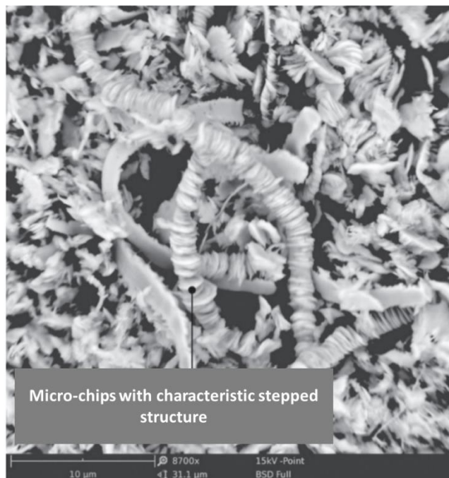
Fig. 9. SEM image of long chips with characteristic stepped construction resulting from micro-smoothing process
