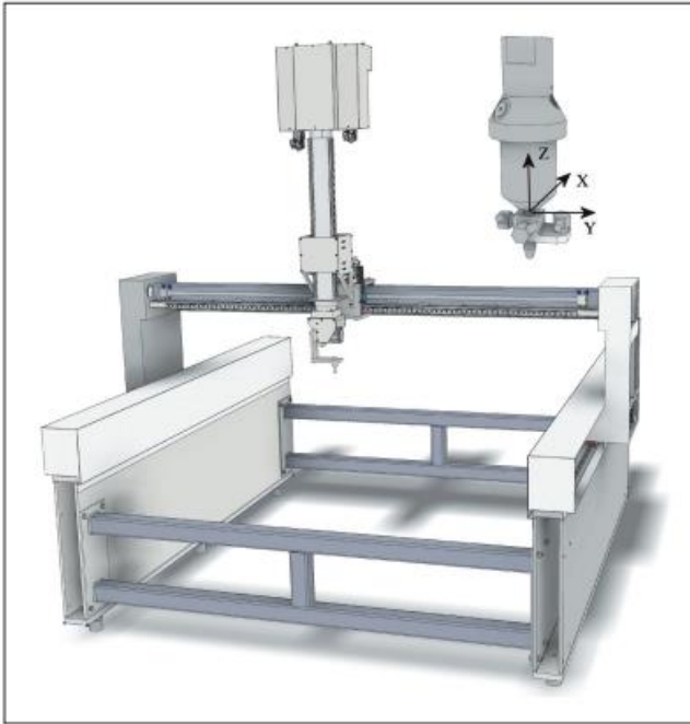
Fig. 1. HWM-P1520/1-3D bearing frame model and the method of fixing piezoelectric accelerometers together with the adopted coordinate system (compatible with the machine axes)
