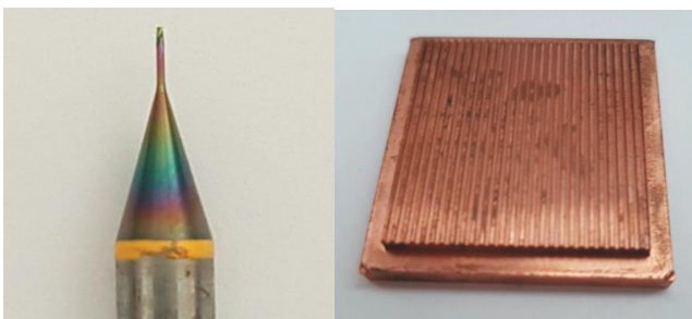
Fig. 1. VHM precision micro milling cutter with DLC coating and the radiator produced by it
