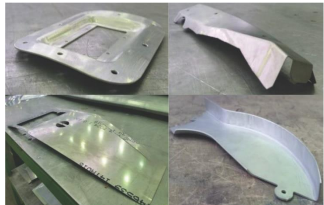
Fig. 1. Examples of products extruded with elastic stamps
