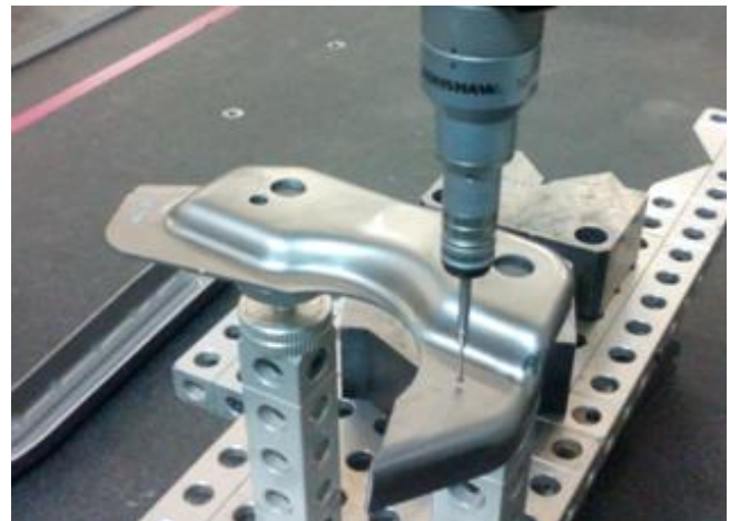
Fig. 9. Working space of the measuring machine during the measurements of dimensional displacement of the extrudate
