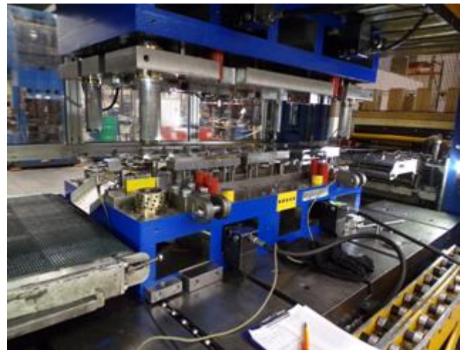
Fig. 5. View of the drawing tool built in crank press with additional equipment
