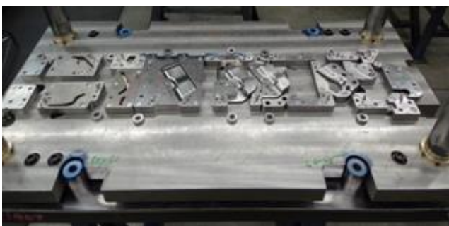
Fig. 3. Upper part of the drawing tool with visible stamps and raised clamp
