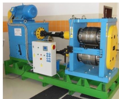
Fig. 5. Prototype roll forging mill for longitudinal and transverse rolling as well as waste-free splitting
