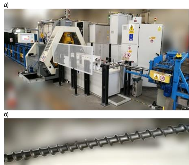
Fig. 4. Automatic technological line for hot screw rolling (a) and finished product (b)
