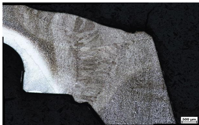
Fig. 1. Macro photograph of the EBW weld (50× magnification)
