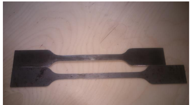
Fig. 5. Not damaged sample (above) and after stretch (below)
