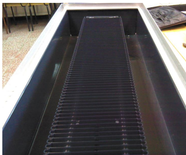
Fig. 1. Channel convection heater subjected to tests
