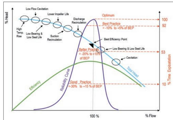
Fig. 1. Pump curve sensitivity for pump reliability [5, 6]
