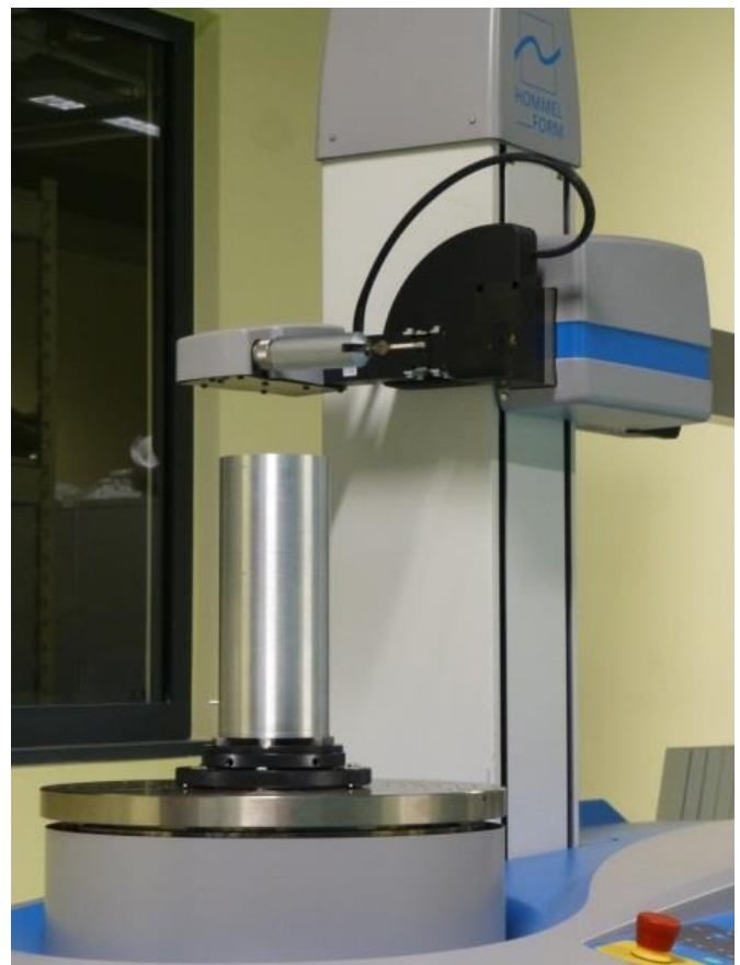
Fig. 1. Jenoptik Hommel Roundscan 535 formtester with measured sleeve (PUT laboratory)
