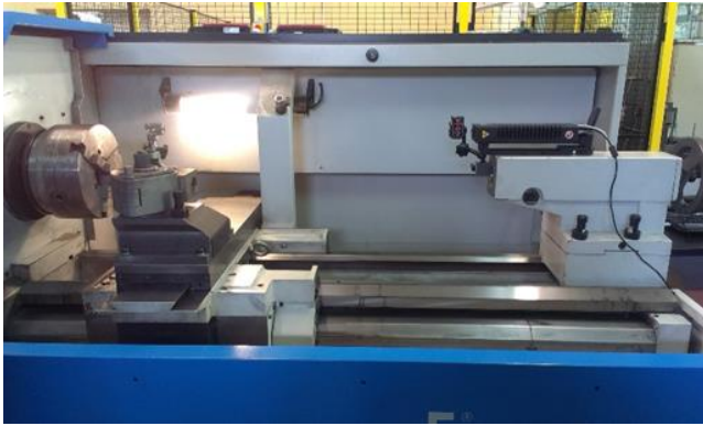
Fig. 1. Attaching the interferometer on the machine tool
