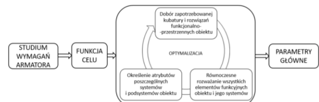
Fig. 2. The scheme of concurrent design based on [10]
