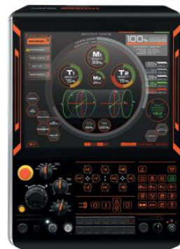
Fig. 6. Smart Box platform and the latest Mazatroll Smooth X driver (source: www.mazak.com)
