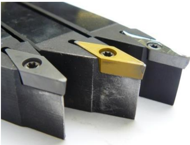
Fig. 8. View of the cutting tools' blades after cutting the worm's coil
