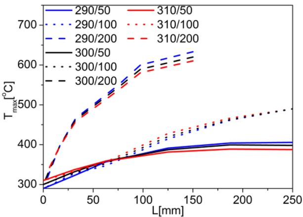
Fig. 6. Increase in the maximum temperature  $T_{max}$  in the inlet duct with a diameter of  $\varnothing 6$  mm on the road  $L$  for PC at different values  $T_m/v$
