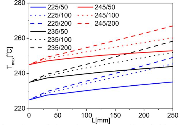
Fig. 10. Increase in the maximum temperature  $T_{max}$  in the inlet duct with a diameter of  $\varnothing 8$  mm on the road  $L$  for PP at different values  $T_m/v$
