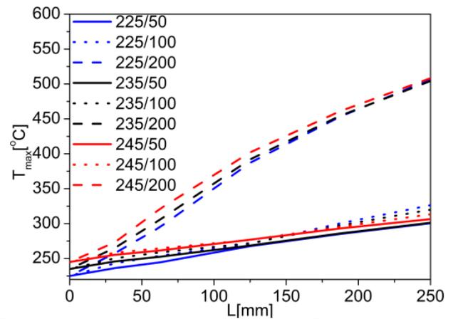
Fig. 8. Increase in the maximum temperature  $T_{max}$  in the intake duct with a diameter of  $\varnothing 4$  mm on the road  $L$  for PP at different values  $T_m/v$
