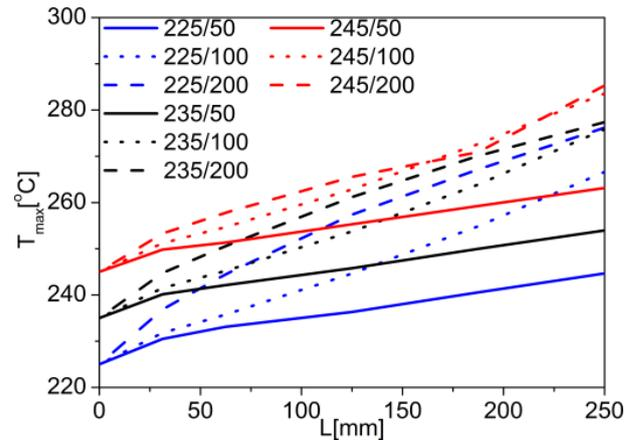
Fig. 9. Increase in the maximum temperature  $T_{max}$  in the inlet duct with a diameter of  $\varnothing 6$  mm on the road  $L$  for PP at different values  $T_m/v$
