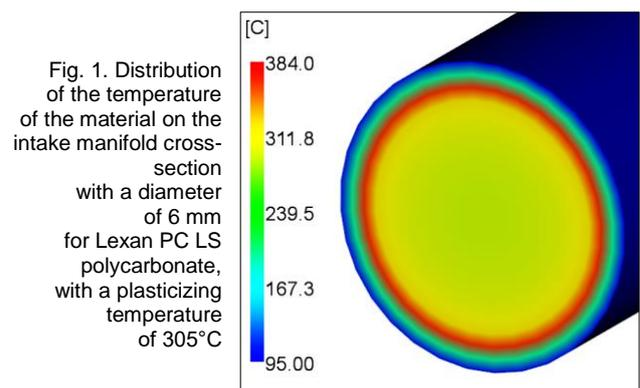
Fig. 1. Distribution of the temperature of the material on the intake manifold cross-section with a diameter of 6 mm for Lexan PC LS polycarbonate, with a plasticizing temperature of 305°C
