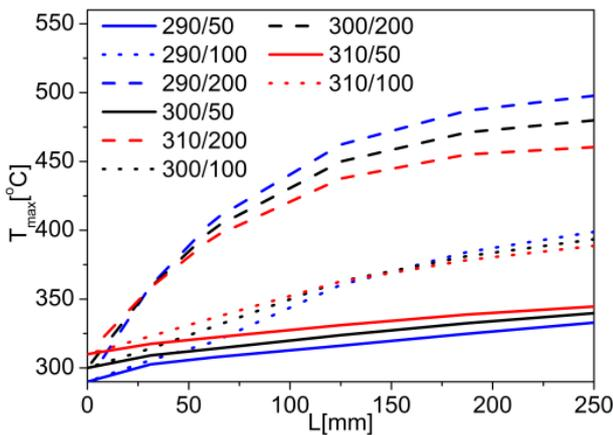
Fig. 7. Increase in the maximum temperature  $T_{max}$  in the intake channel with a diameter of  $\varnothing 8$  mm on the road  $L$  for PC at different values  $T_m/v$
