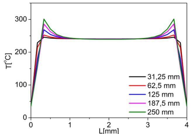
Fig. 4. Distribution of temperature  $T$  of PP material on the cross-section of the inlet channel along the channel diameter for different flow path
