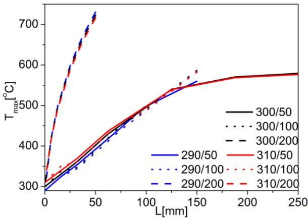
Fig. 5. Increase in the maximum temperature  $T_{max}$  in the intake duct with a diameter of  $\varnothing 4$  mm on the road  $L$  for PC at different values  $T_m/v$
