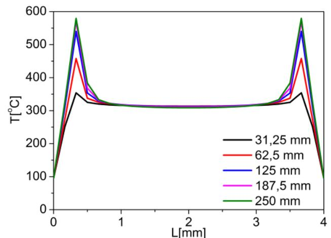
Fig. 3. Temperature distribution  $T$  of the PC material on the cross-section of the inlet channel along the channel diameter for different flow path
