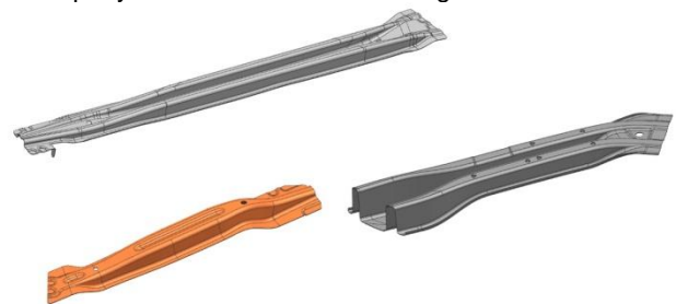
Fig. 2. Typical constructions of door reinforcing beams
