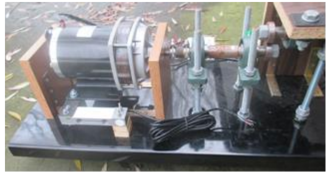
Fig. 3. View of mounting the extensometer beam to the plate and drive motor
