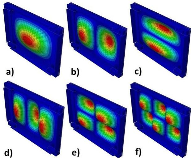
Fig. 10. Six first forms of natural vibrations (description in the text)
