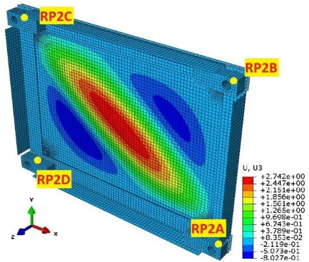
Fig. 9. Map of displacements in the direction perpendicular to the plate
