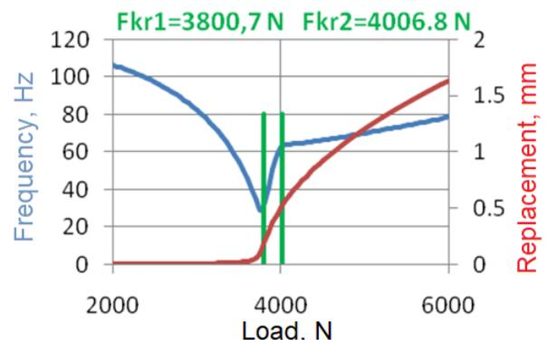
Fig. 11. Dependence of frequency and displacements on the load
