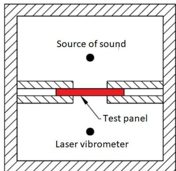
Fig. 1. Measurement scheme
