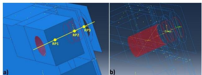
Fig. 6. Way of modeling the bolt connection in FEM
