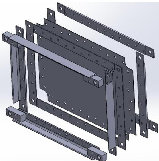
Fig. 4. Panel – exploded view without connecting elements
