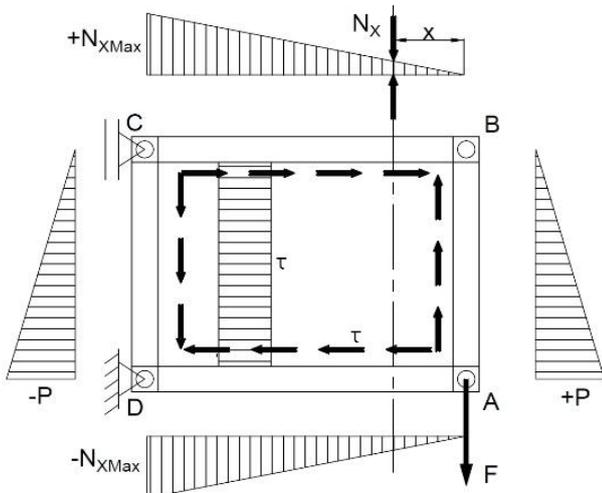
Fig. 2. Panel model – loads and boundary conditions
