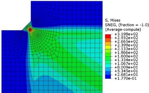
Fig. 7. Map of stresses reduced in MPa in the corner C of the slab
