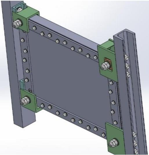
Fig. 3. Construction of the panel with restraints
