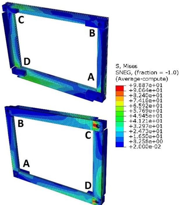
Fig. 8. Map of reduced stresses according to the Huber-Mises-Hencky hypothesis in the skeleton elements
