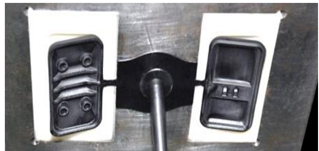
Fig. 1. Injection mold with inserts made by the MJM method on the 3D systems machine [6]
