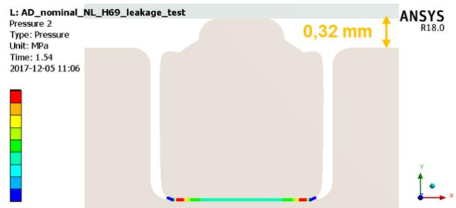
Fig. 5. Pressure in contact in the critical area of the seal
