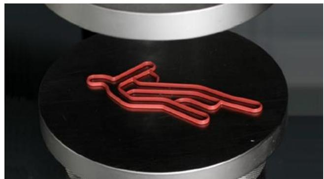
Fig. 1. Tested seal between plates of a durability machine (photo: Tomasz Pietrzak)
