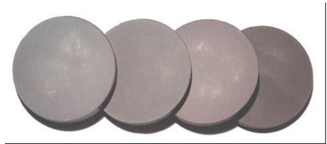
Fig. 4. Samples of ceramic materials for EDM treatment after sintering with the SPS method
