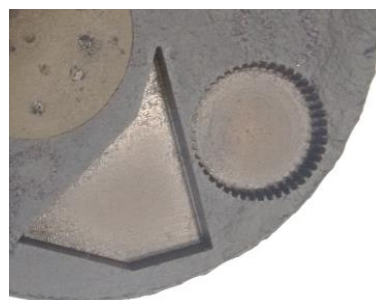
Fig. 8. EDM shaped molds in \text{Al}_2\text{O}_3\text{-Ti(C,N)-TiB}_2 composite
