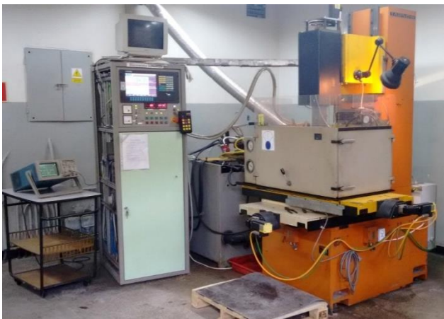
Fig. 5. Experimental EDEF-40 EDM machine
