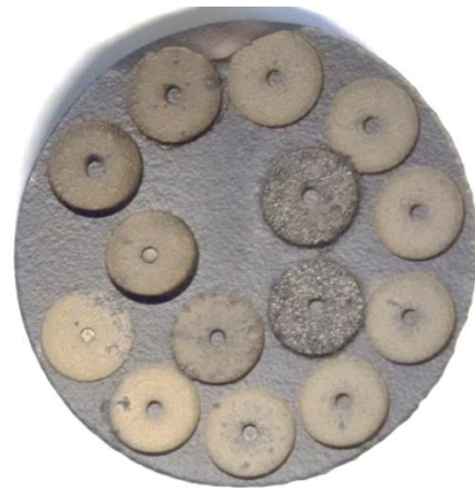
Fig. 6. Al 2 O 3 -Ti(C, N) - TiB 2 composite with molds
