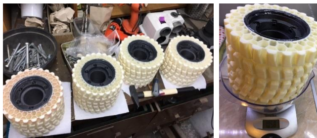
Fig. 8. Ready wheels of the KALMAN rover
