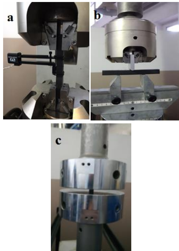
Fig. 3. PETG material reinforced with carbon fiber: a) tensile strength test with extensometer, b) flexural strength test, c) compression test
