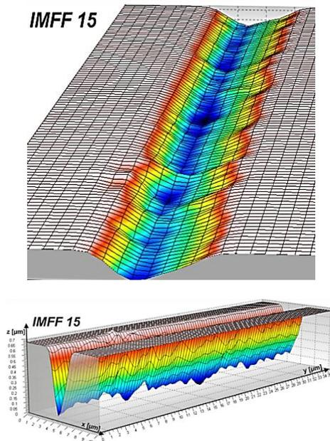
Fig. 5. Fragment of the micro-cutting trace with visible unevenness of the bottom of the crack and with the grain of an electrocorund attached to the surface of the abrasive film 15 IMFF
