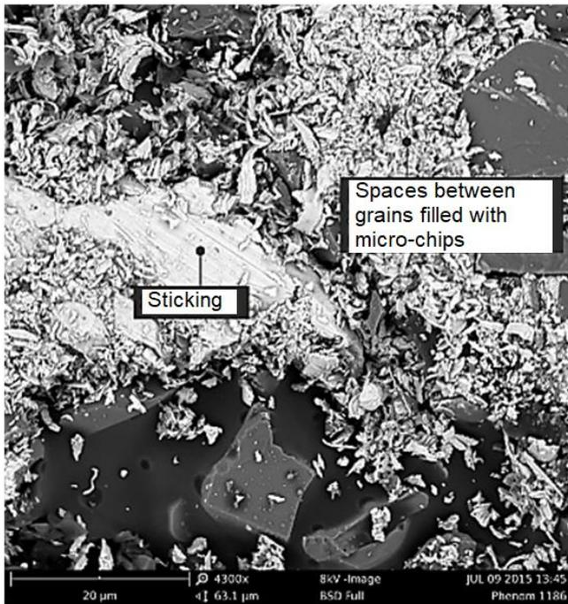
Fig. 2. SEM image of IMFF abrasive foil 15 after a micro-smoothing process with visible adhesion and microbial spaces filled with grains
