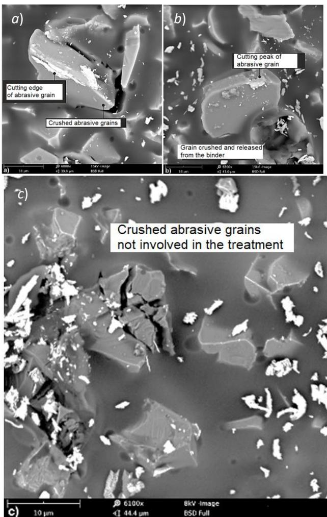
Fig. 3. SEM image of IMFF abrasive foil 15 after the micro-smoothing process: a) with visible broken grain after micro-smoothing, b) with grain crushed and released from the binder, c) with crushed grain
