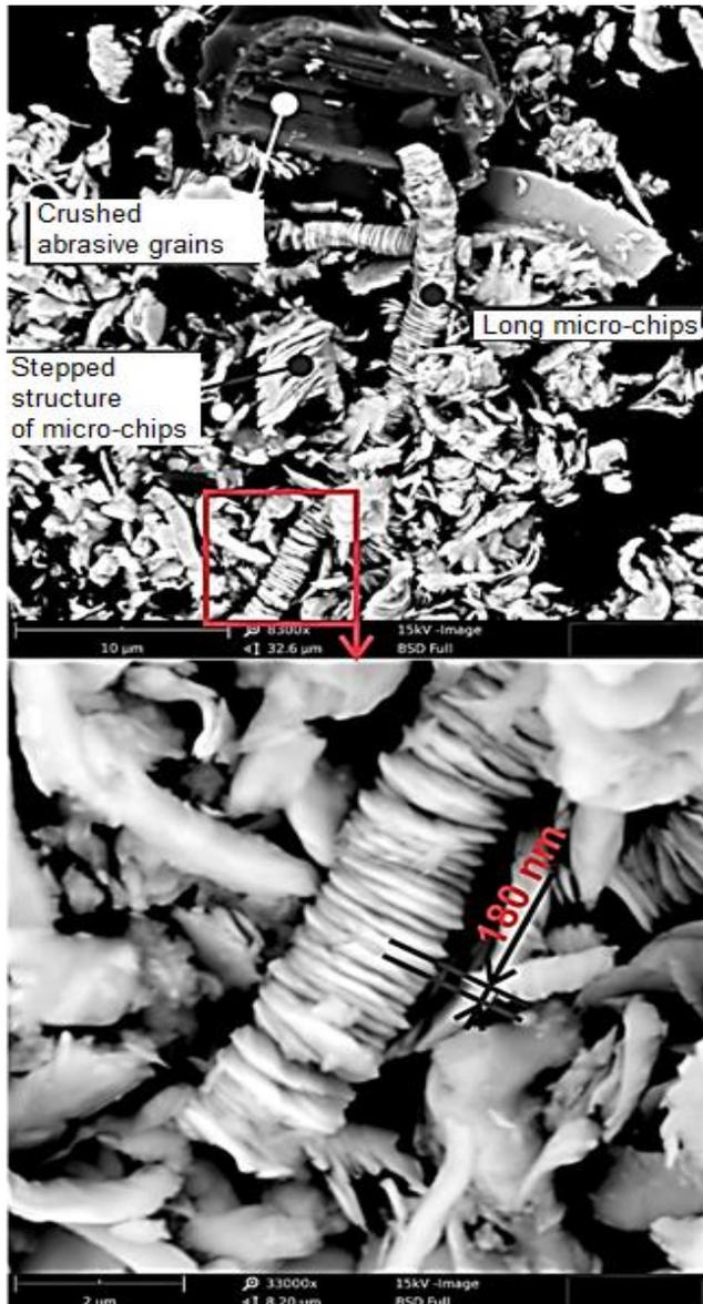
Fig. 6. SEM images of microflora resulting from the micro-smoothing process of 40H steel with stepped construction and plate thickness of 180 nm
