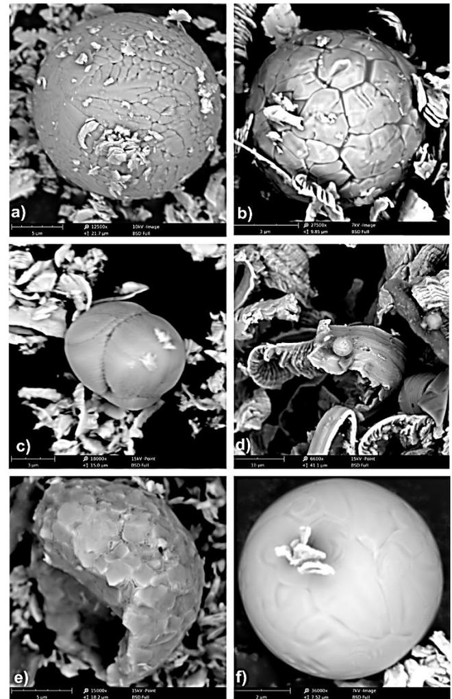
Fig. 4. SEM images of spherical microspheres after the micro-smoothing process: a) with visible very complex surface structure, b) with a surface made of large, geometric elements, c) with a shape deviating from the sphere, d) with a characteristic stepped structure, glued to the surface e) made up of small elements that make up a fragment of the sphere, f) with a very smooth surface
