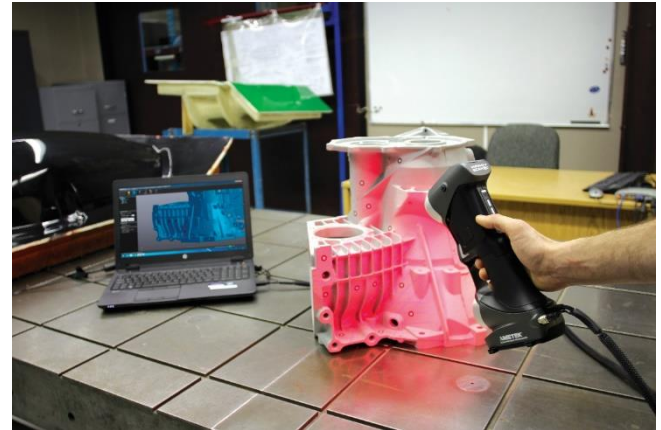
Fig. 3. HandySCAN 700 portable laser scanner when scanning a cast [6]
