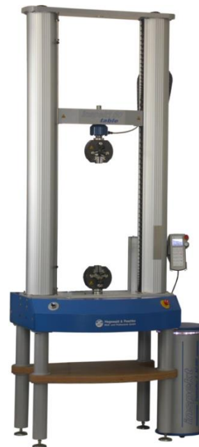
Fig. 2. Inspekt table 50 kN testing machine for calibration of technological devices (e.g. dynamometers) in the customer's premises or in the ITA laboratory
