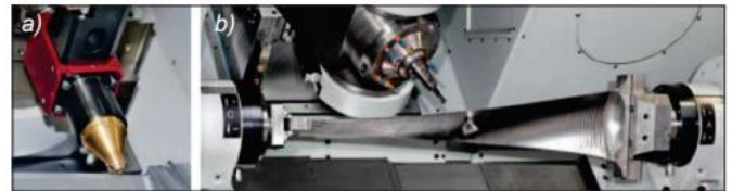
Fig. 17. Edge deposition (a) and milling of the turbine blade after deposition (b) [21]
