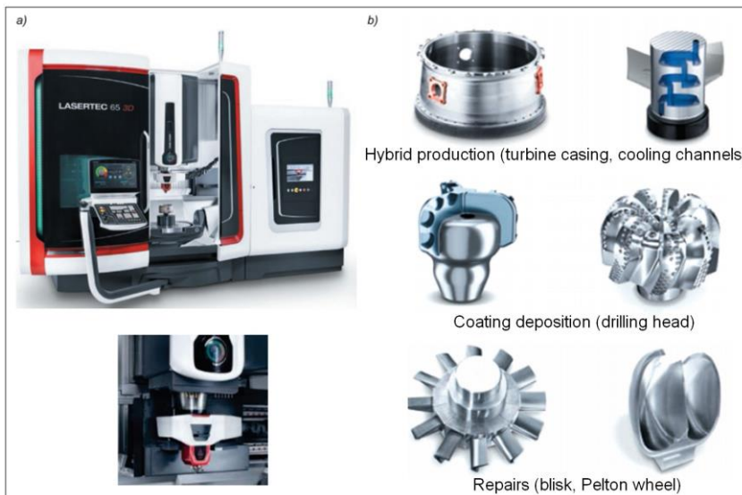
Fig. 18. Integration of a five-axis milling machine with laser cladding (a) and examples of application (b) [7]
