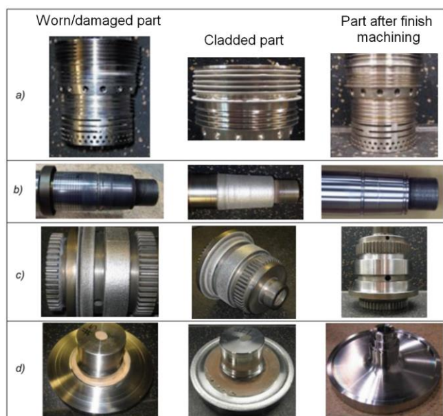
Fig. 19. Examples of repairing various products using the LDT technique [18]: a) repair of the gas compressor housing (material: Inconel 718), b) repair of the steel shaft 4340 (welded material: corrosion resistant steel 420 LC), c) repair of the planetary gear connector (welded material: 420 LC corrosion resistant steel), d) repair of undersized forgings (welded material: Ti6-4 titanium alloy)
