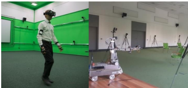
Fig. 2. Movement of the person taking part in the research (left) will be transferred to the appropriate movement of the robot in the adjacent room (on the right)
