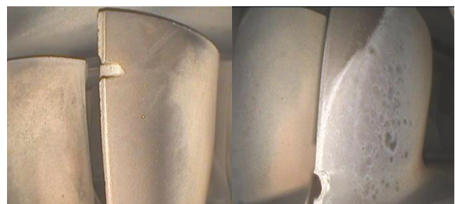
Fig. 1. Exemplary damages of air compressor blades of a turbine engine
