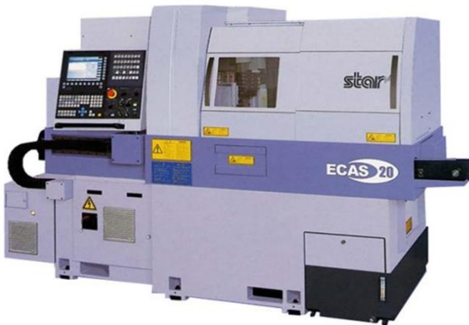
Fig. 6. Star ECAS-20 longitudinal automatic machine [7]
