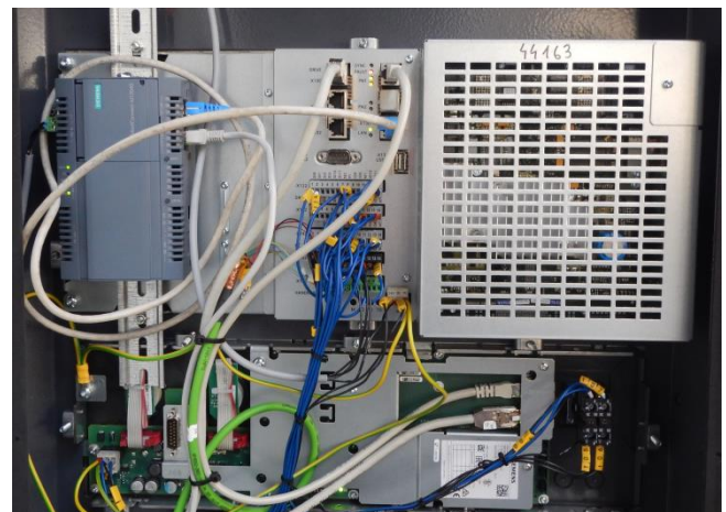
Fig. 3. MindConnect IoT 2040 installed with the SINUMERIK 828D controller
